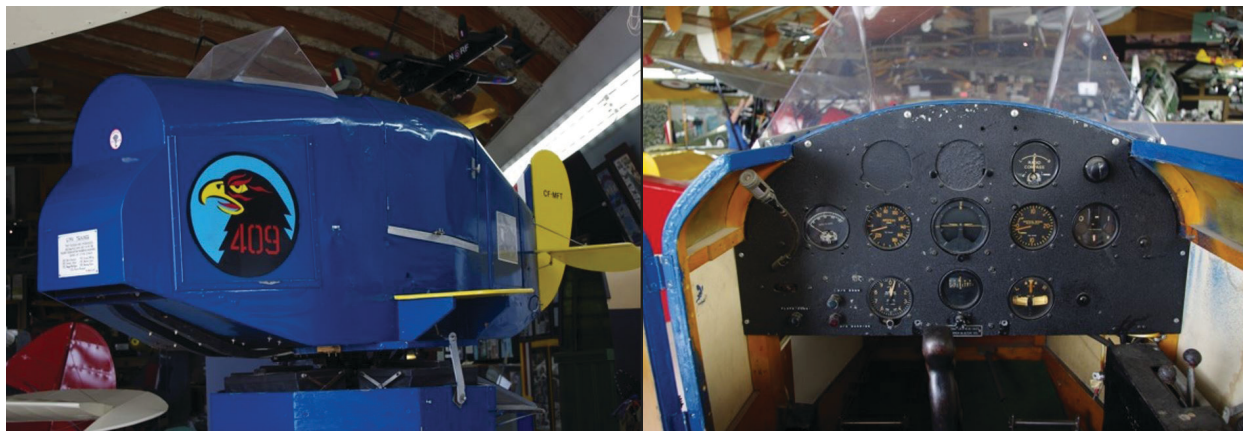
Figure 73. The blue Link trainer and it's instrument panel. – photo courtesy Canadian Museum of Flight
